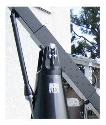
Changing the Boom arm is as simple as lifting the handle on each side at the top of the cone and removing the pin from the top of the lift tube. The Boom arm is lifted out and the size needed is put back in its place.
