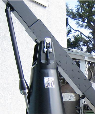
Changing the Boom arm is as simple as lifting the handle on each side at the top of the cone and removing the pin from the top of the lift tube. The Boom arm is lifted out and the size needed is put back in its place. Reverse the procedure above and you are done!
